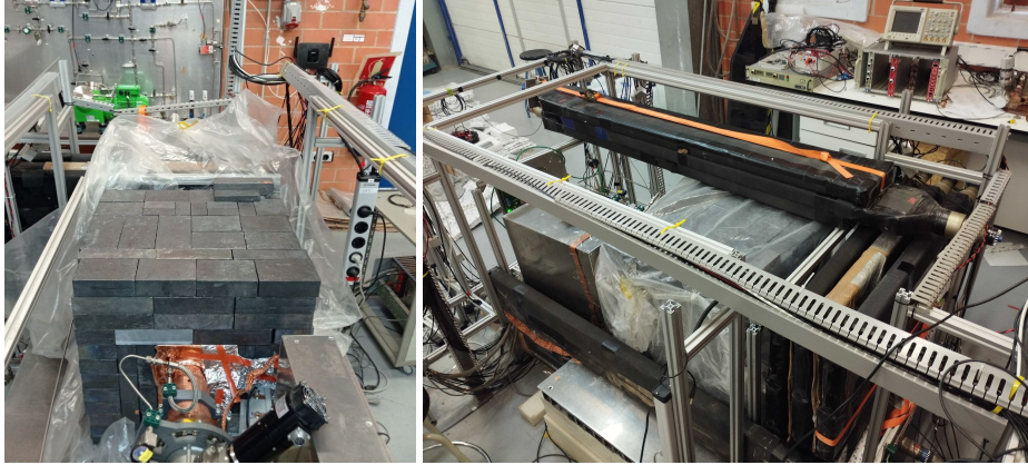
Figure 3.5: IAXO-D1 setup at the CAPA IAXOLab. Left: Picture showing the inner passive shielding composed by 20 cm of lead. Right: Picture with part of the active shielding composed of plastic scintillators installed.
