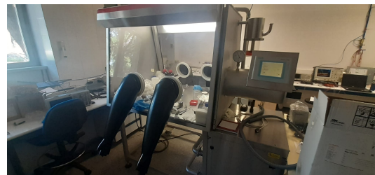
Figure 8.5: Picture of the ANAIS glove box, continuously keeping a dry atmosphere to preserve and work with sodium iodide crystals.
