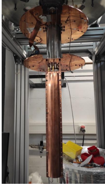
Figure 3.19: Picture of the 10\times scaled-down prototype of BabyIAXO cavity made on copper, just manufactured and tested in 2024.
