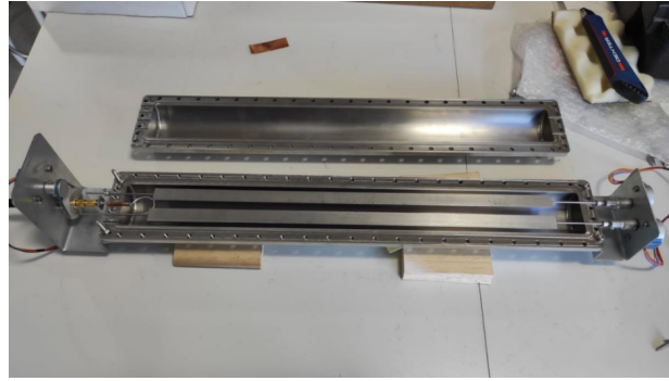
Figure 3.18: Picture of the 10\times scaled-down prototype of BabyIAXO cavity, just manufactured and tested in 2023.
